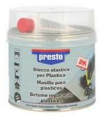
presto Putty for plastics is a 2-component black polyester putty as a mixture of a highly elastic, amino-preaccelerated polyester resin with different mineral, environment-friendly fillers. To fill scratches and damages and to aftertreat bonded plastic parts. Through its thixotropy and softness, profiles and contours can easily be rebuilt
