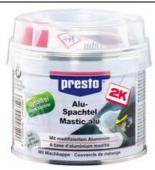
presto Aluminium Putty "styrene-free" is a 2-component polyester filling putty as mixture of a medium-elastic, highly reactive, amino-preaccelerated polyester resin with different mineral, environment-friendly fillers and aluminium pigments.
