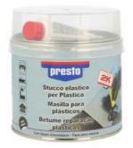
presto Putty for plastics is a 2-component black polyester putty as a mixture of a highly elastic, amino-preaccelerated polyester resin with different mineral, environment-friendly fillers. To fill scratches and damages and to aftertreat bonded plastic parts. Through its thixotropy and softness, profiles and contours can easily be rebuilt.
