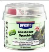
presto Glass Fibre Filler is a 2-component polyester putty containing the new adhesion promoter NT. The putty is a mixture of pure, unsaturated polyester resin and glass fibre particles. Applicable in industry and DIY sector for bigger damages, which are perforated by corrosion and which are exposed to special mechanical stress. Suitable for application on metal, wood, concrete and many plastics etc.
