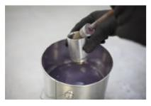
**Step 12:** Clean the Teflon piston and metal cylinder thoroughly with appropriate solvent.
