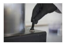
**Step 9:** During the filling process the switch should stay for one to two seconds. If this is shorter (depends on viscosity) you can extend the time by holding the switch.
