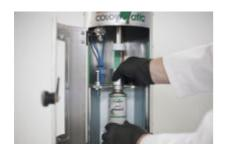
**Step 6:** Put the spray can and cylinder on the distance adapter and push up against it with both hands into the machine.
