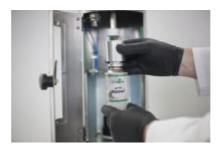
**Step 10:** After completion the filling process, open the door. Take out spray can and cylinder.
