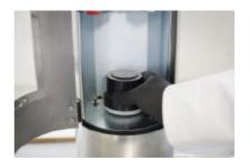
**Step 5:** Put the distance adapter on the can plate.
