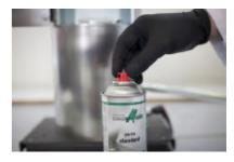
Step 10: Put on the nozzle immediately with a slight rotation.
