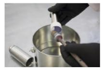
Step 11: Clean the Teflon piston and metal cylinder thoroughly with appropriate solvent.
