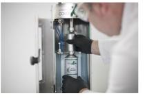
**Step 13:** After completion the filling process, open the door. Take out spray can and cylinder.
