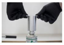
**Step 4:** Insert the CleanJector with a slight quarter rotation
