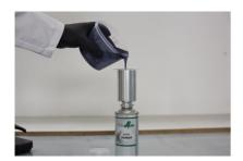
Schritt 6: Pour the colour into the CleanJector.
