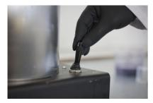
**Step 12:** During the filling process the switch should stay for one to two seconds. If this is shorter (depends on viscosity) you can extend the time by holding the switch.
