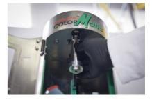
**Step 8:** Take off the white teflon piston and Insert metal piston
