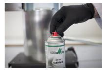
**Step 14:** Put on the nozzle immediately with a slight rotation.
