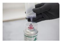
**Step 15:** You can mark the cap with the drop which remains on the cone end of the CleanJector.
