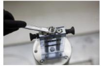
**Step 8:** A vernier adjustment is possible with a screw-wrench no. 17.
