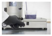
**Step 10:** Turn the switch to "suction" – the colour will be drawn into the machine. Depending on the viscosity of the lacquer takes it more time.
