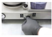
**Step 9:** With the switch on the front you can choose either the position "suction" (on the right) or "filling" (on the left).
