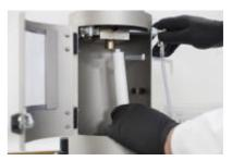
**Step 2:** Put the bar between filler neck and can plate.
