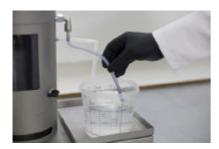
**Step 1:** Instead of the varnish container put a container with to the filled lacquer suitable solvent under the suction hose.
