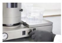
**Step 5:** Turn the switch to suction". The solvent will be sucked.
