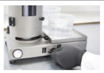
**Step 6:** Then switch to position "filling". Because the filling is blocked, the contaminated solvent will be conducted into the collecting tray.
