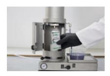
**Step 12:** Open the door, take out spray can. The filling machine is now ready to fill more spray cans with the same lacquer.
