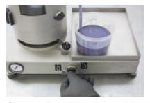
**Step 11:** Turn the switch to "filling" – the lacquer will be pressed into the spray can.
