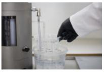
**Step 4:** Close the door and take under the second hose a collecting tray for the contaminated solvent. Insert the hose.
