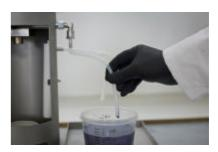
**Step 2:** Put the container with varnish on the bin and insert the suction hose.
