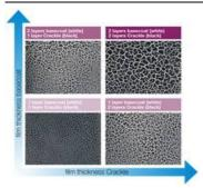
Tuning Crackle Effect is a 2-coat effect spray. It produces on different acrylic- or nitro-combi surfaces looking as if torn up, e.g. like leather. So it creates a very effective look.
