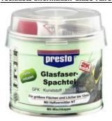
presto Glass Fibre Filler is a 2-component polyester putty containing the new adhesion promoter NT. The putty is a mixture of pure, unsaturated polyester resin and glass fibre particles. Applicable in industry and DIY sector for bigger damages, which are perforated by corrosion and which are exposed to special mechanical stress. Suitable for application on metal, wood, concrete and many plastics etc.
